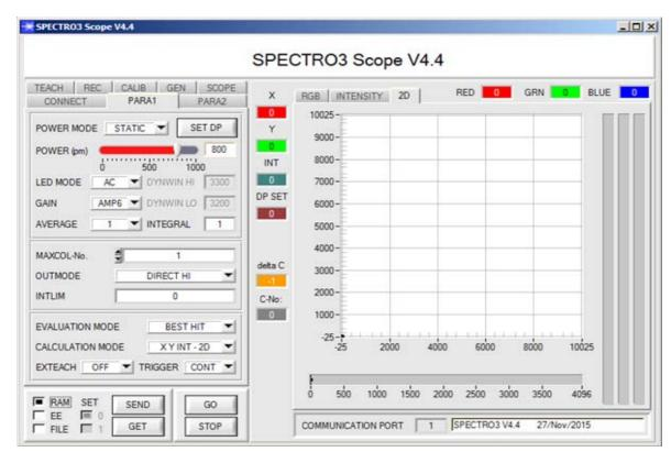
Under Windows® representation of the color value on a PC in numeric form and in a color chart, and representation of RGB values in a time chart. In addition the current RGB values are displayed as a bar chart.
