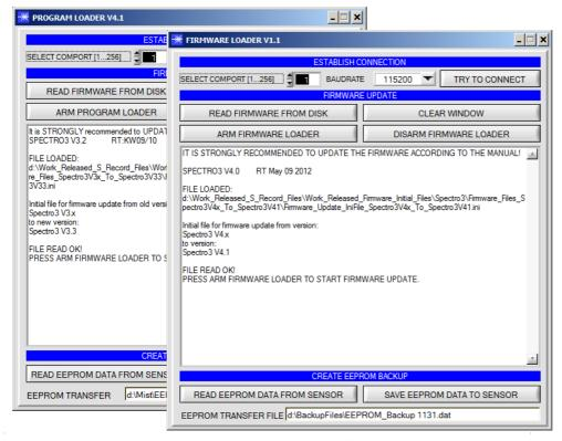
The software "ProgramLoader" or "FirmwareLoader" allows the user to perform an automatic firmware update. The update will be carried out through the RS232 interface.
