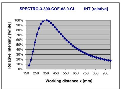
Relative intensity SPECTRO-3-300-COF-d8.0-CL: 100% at a working distance of 360 mm (INTENSITY 3264)
