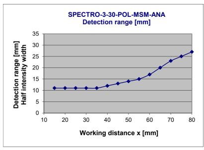
Relative intensity SPECTRO-3-30-POL-MSM-ANA: 100% at a working distance of 15 mm (INTENSITY 3703)
