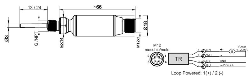
IO-Link: 1(+) / 3 (GND) / 4 (IO-Link) Switch.Out: 1(+) / 3 (GND) / 4 (Out)
