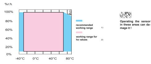
1) In continuous operation mode, the elements should be used up to an absolute humidity level which corresponds to a dew-point temperature not exceeding 60°C. The elements can be used at dew-point temperatures of up to 90°C during short work cycles (e.g. in a control process).
