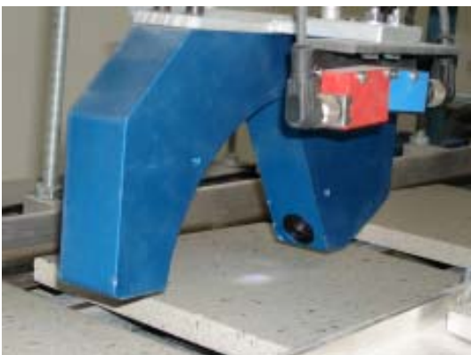
Gloss degree monitoring at plates of stone
