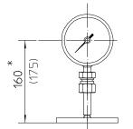
\*The necktube is extended by 36 mm for thermometers without capillaries and with scale ranges ≥160°C
